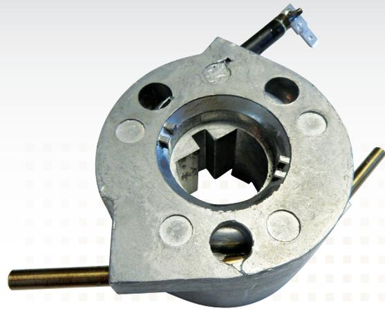
The manufacturer needed to design and create a heater block for coffee maker stands. The finished product needed to be high pressure diecast in aluminium. The process wasn't straightforward because the casting had integrated electrical pipework and water pipes coiled throughout the product, making it more complicated.
